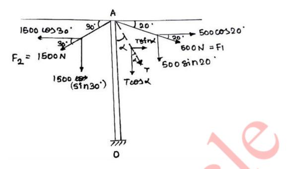
Given:- In the figure , F1=500N,F2=1500N,T=?,F1 makes an angle 20° with horizontal and F2 makes 30° with the horizontal and assume tension 'T' makes an angle  $\alpha$  with vertical.
